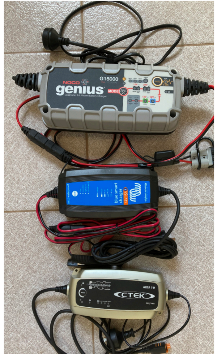
Figure 4. Some examples of smart chargers. It is important you buy something that suits the types of batteries you have (e.g. flooded lead acid, AGM, Gel, lithium) and is large enough for your largest battery. Remember the 10% rule (as a rule of thumb your battery charger should be a minimum of 10% of the Ah rating of the battery, e.g. A 100Ah battery would require a 10 Amp charger as a minimum).
