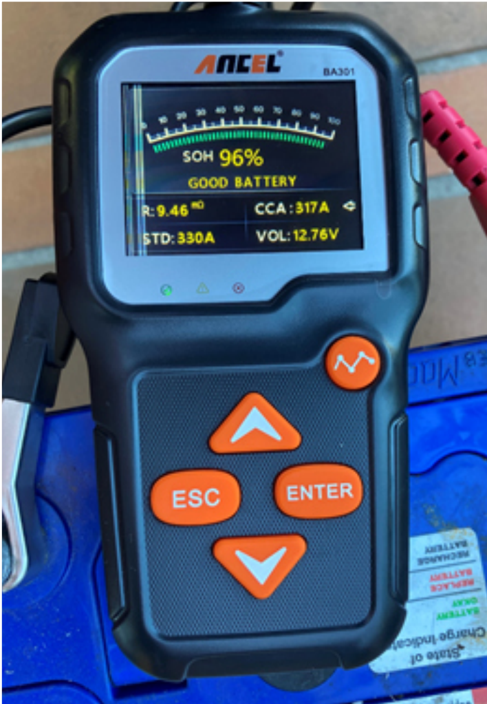
Figure 3. Analysis results showing IR of 9.46 milliohm, CCA 317A and voltage of 12.76V leading to the assessment that the battery condition was good. SOH is state of health or percentage charge. The STD is the rated CCA of the battery which you enter into the analyser prior to use.
